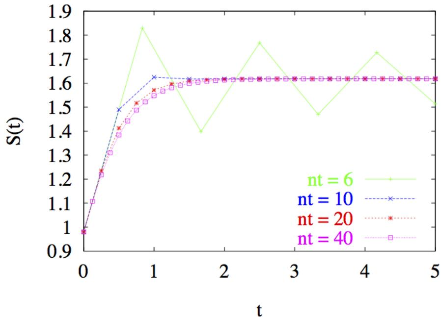
**Figure Saturation Time Series:** Plot of the saturation ratio as a function of time using the Forward Euler method. “nt” is the number of time steps.
