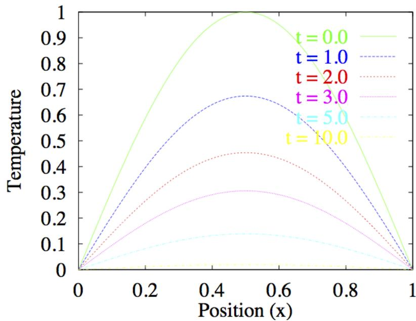
**Figure 1d-diffusion** Temperature vs. position curves at various times, for heat diffusion in a rod with sinusoidal initial temperature distribution and parameter value  $\alpha = 0.2$ .
