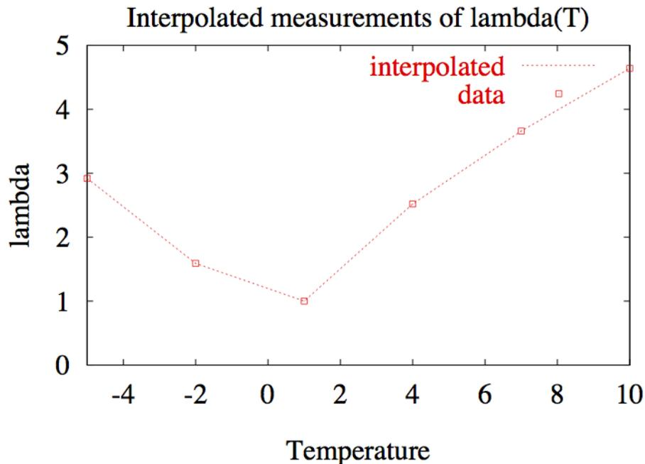
**Figure Table:** A rock with  $\lambda$  known only at a sequence of discrete temperature values, from experimental measurements. The function  $\lambda(T)$  can be represented approximately using linear interpolation (and the resulting approximate function can then be used to solve the problem numerically).
