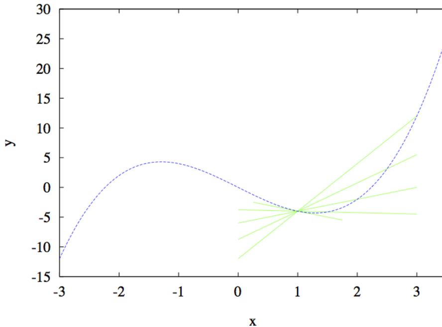
**Figure Tangents:** Plot of the function  $y = x^3 - 5x$  and the forward difference approximations to the derivative for various values of  $\Delta t$
