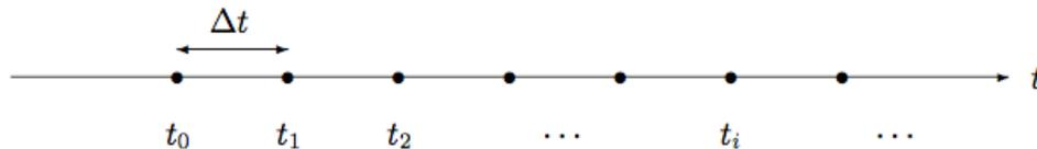
**Figure Grid:** A grid of equally-spaced points,  $t_i = t_0 + i\Delta t$ , for  $i = 0, 1, 2, \dots$
