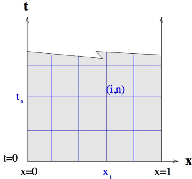
**\*\*Figure PDE Grid:\*\*** The computational grid for the heat diffusion problem, with discrete points  $(x_i, t_n)$ .
