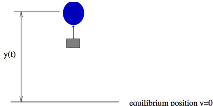
**Figure Weather Balloon:** A weather balloon oscillating about its level of neutral buoyancy.
