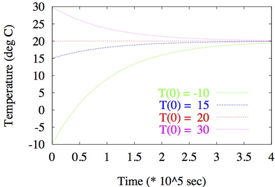
**Figure: Conduction** Plot of solution curves  $T(t)$  for  $T_0 = -10, 15, 20, 30$ ; parameter values:  $\alpha = 10^{-5}$ ,  $T_a = 20$ .
