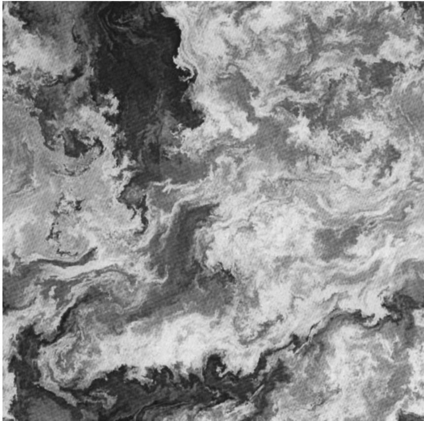
Figure 10 A snapshot of the spatial amplitude of an evolved scalar field from the direct numerical simulations of Chen & Kraichnan (1998) using a white noise velocity field. White is warm. Black is cool. Although the white noise calculations are inconsistent with the scaling exponent for the scalar structure functions determined by experiment (see text), they do capture the qualitative characteristics of the small scale intermittency, and of the ramp-cliff structures (which occur along the lines of demarcation between the warm and cool fluid).
